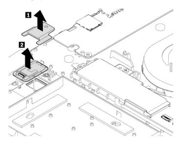
9. Install the new fingerprint reader and the bracket in place.
