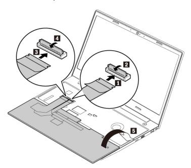
2. Insert the keyboard into the keyboard bezel as shown. Ensure that the front edge of the keyboard (the edge that is close to the display) is under the keyboard bezel.
