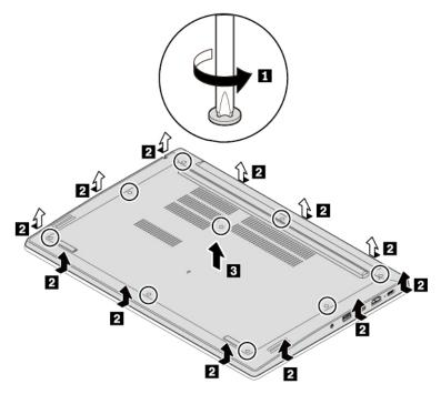
5. Install the new base cover assembly **11** and ensure that the latches of the base cover assembly are secured in place 2. Then tighten the screws 3.
