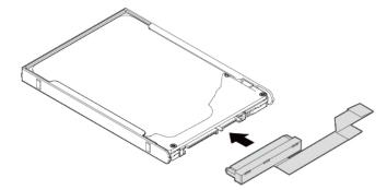
3. Insert the new hard disk drive together with its bracket and pivot it downward. Ensure that the new hard disk drive is seated in place. Connect the hard-disk-drive cable to the system board.
