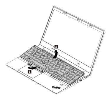
10. Put the keyboard on the palm rest as shown and detach the connectors. Then remove the keyboard.
