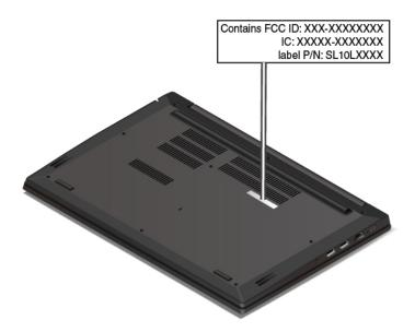
For a factory-preinstalled wireless module, this label identifies the actual FCC ID and IC certification number for the wireless module installed by Lenovo.
