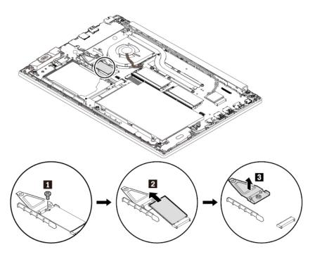
8. Install the short bracket in place 1. Insert the new M.2 solid-state drive into the slot at an angle of about 20 degrees 2 and pivot the M.2 solid-state drive downward 3. Install the screw 4 to secure the M.2 solid-state drive.
