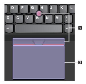
By default, both the TrackPoint pointing device and the trackpad are active with the touch gestures enabled. To change the settings, see "Customizing the ThinkPad pointing device" on page 19.
