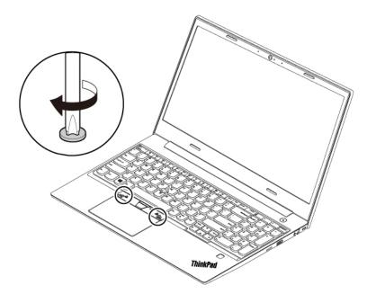
5. Take the new TrackPoint buttons out of the new keyboard package. Install the TrackPoint buttons as shown.
