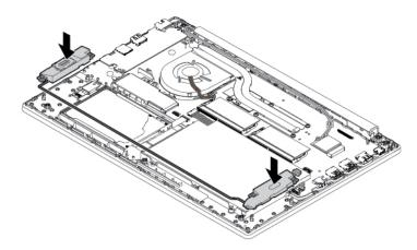
8. Attach the connector of the speaker assembly.
