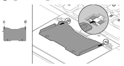
8. Pivot the tool in the direction as shown to release the keyboard . Push the keyboard in the direction as shown by arrows 2 to release the latches from the keyboard bezel.
