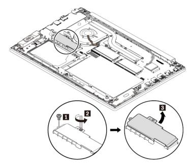
7. Remove the screw 1 and remove the short M.2 solid-state drive 2. Remove the short bracket if you want to replace it as well 3.
