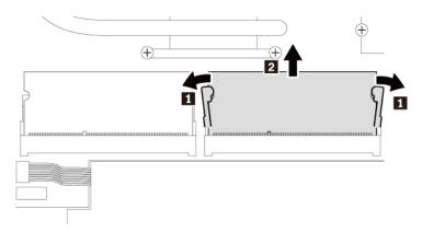
6. Insert the new memory module into the memory slot at an angle of about 20 degrees . Pivot the memory module downward until it snaps into place . Ensure that the memory module is firmly installed in the memory slot and cannot be moved easily.
