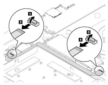
6. Remove the cable as shown.
