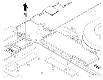
8. Remove the bracket and the fingerprint reader.
