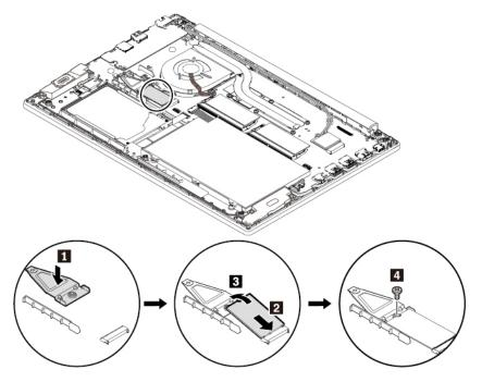
9. Install the long bracket as shown 1 2. Install the screw 3 and tighten the screw 4.
