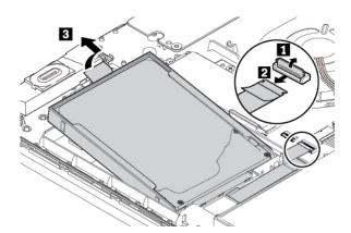
6. Detach the cable from the hard disk drive.
