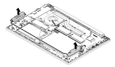
7. Install the new speaker assembly in place.
