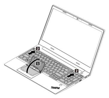
9. Pivot the keyboard slightly upward as shown by arrow 1. Then turn the keyboard over as shown by arrow 2.
