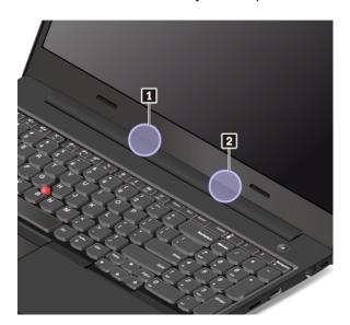
Wireless-LAN antenna (auxiliary)Wireless-LAN antenna (main)
