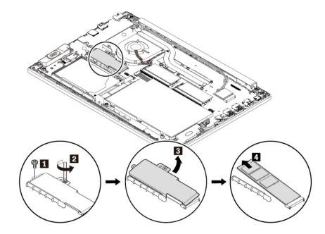
7. Insert the new M.2 solid-state drive into the slot at an angle of about 20 degrees 11 and pivot the M.2 solid-state drive downward 2. Then, reinstall the bracket into place as shown 3 4. Install the screw 5 and tighten the screw 6.
