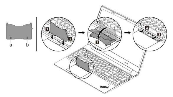
6. Loosen the screws that secure the keyboard.
