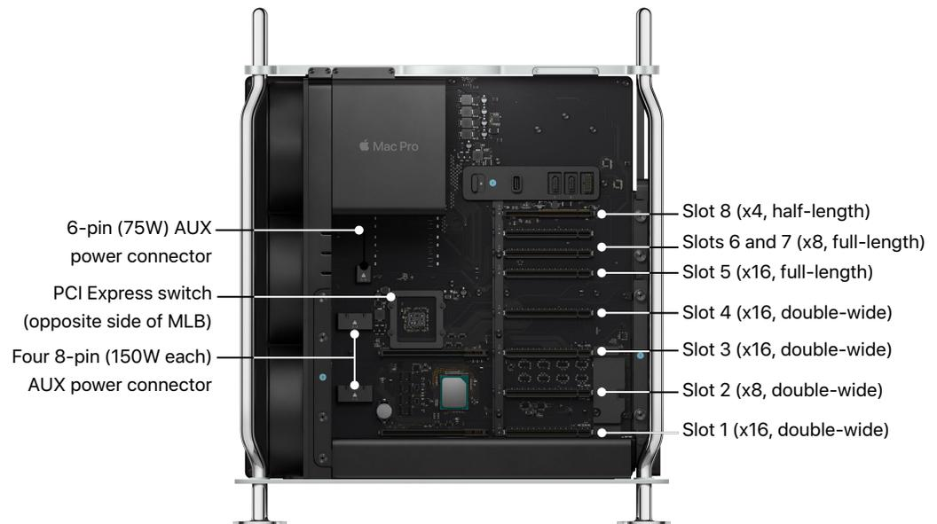
Mac Pro provides four 8-pin auxiliary (AUX) power connectors that each provide 150W of power, for a total of 600W of AUX power. This power is in addition to the 75W of power provided directly by each PCIe slot. Combined, up to four 225W graphics cards can be installed in Mac Pro, each in an x16 slot with a total power of 900W. A single 6-pin AUX power connector provides 75W of additional power for PCIe cards in slots 5, 6, and 7.
