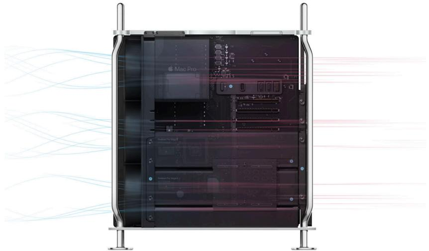
The extreme performance of Mac Pro requires a tremendously capable thermal system. Three axial fans quietly push air across the CPU and the GPUs, keeping them cool under even the most intensive workloads. On the opposite side, a blower pulls the air across the memory and storage and through the power supply, exhausting it out the back of the machine.
