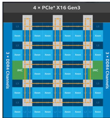
Workstations require high-bandwidth connectivity to compute, graphics, and storage resources inside the system. This new generation of Intel Xeon W features 64 PCI Express lanes for massive bandwidth in and out of the processor.
