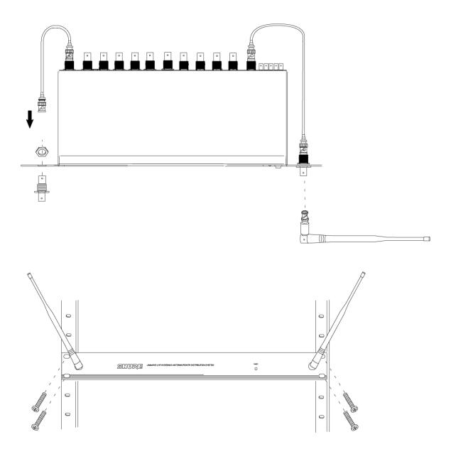
Installation and Cable Connections
