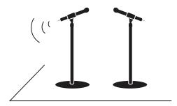
**Important:** Always perform a "walk around" test to verify coverage before using a wireless system during a speech or performance. Experiment with antenna placement to find the optimum location. If necessary, mark "trouble spots" and ask presenters or performers to avoid those areas.
