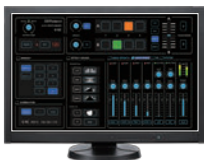
If you set the preview output to Preview mode, you can switch the program output(A Bus) video and the preview output(B Bus) video respectively. *Transition effects can not be applied in this mode.
